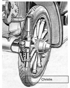
Christie used a pillar sliding through upper and lower supports which were extensions fixed to each side of the front of the chassis. A helical coil spring surrounded the pillar and on some examples there seems to have been a smaller rebound/ snubber spring at the bottom.
