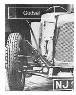
vives in restored form. The suspension, a sliding axle design. had a stub axle which slid on an inner vertical tube with a main spring above it and smaller rebound spring below. This was all
